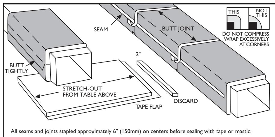
All seams and joints stapled approximately 6" (150mm) on centers before sealing with tape or mastic.
