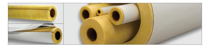
ALLEY-K<sup>TM</sup> is a preformed pipe insulation composed of high quality glass fibres, bonded together with a thermosetting resin. The lightweight, 36" pipe sections are manufactured with the flame attenuated process and are available with or without the all service jacket (ASJ). Our unique wrinkle-free all service vapour retarder jacket (ASJ) reinforced with glass fibres comes with a factory applied pressure sensitive self-sealing lap closure system (SSL). Butt strips are also supplied.
