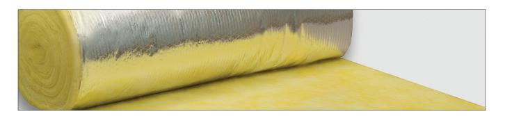
ALLEY WRAP FSK<sup>™</sup> is a lightweight, highly resilient thermal insulation blanket faced with an FSK (foil, scrim, kraft) facing. Manufactured from high quality flame attenutated glass fibres, ALLEY WRAP FSK<sup>™</sup> has excellent thermal and acoustical properties. The extremely fine, long glass fibres are bonded with a thermosetting binder.
