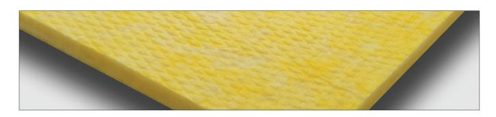
AK BOARD<sup>TM</sup> is a rigid, lightweight board produced from flame attenuated glass fibres. The extremely fine, long glass fibres are bonded with a thermosetting binder. AK BOARD<sup>TM</sup> has excellent thermal and acoustical characteristics. It is available in yellow or black; plain, or with a smooth and rigid glass mat surface (HD).
