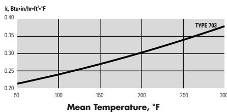
Apparent thermal conductivity curve determined in accordance with ASTM Practice C 1045 with data obtained by ASTM Test Method C 177. Values are nominal, subject to normal testing and manufacturing tolerances.
