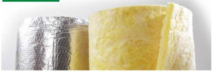
**ALLEY WRAP**® fiberglass blanket insulation is a thermal and acoustical insulation product made from highly resilient, inorganic glass fibers bonded by a thermosetting resin. It is available unfaced or with a multi-purpose foil-scrim kraft (FSK) jacket. Vapor retarders have a 2" (51 mm) stapling flange on one edge, and the factory-applied facing assures uniform quality.
